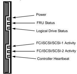
Figure 2. VTrak M300f/i/p and M200f/i/p front panel LEDs
